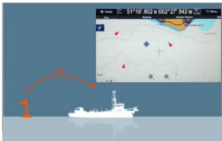
*Correct depiction of an AIS AtoN marking a buoy on an electronic chart display*
