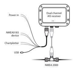
Figure 3 Electrical connections to the AIS receiver
