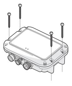
Figure 6 AIS receiver mounting
