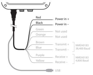
Figure 10 Connecting the power supply
