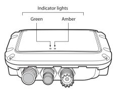
Figure 11 Indicator location on the AIS receiver unit
