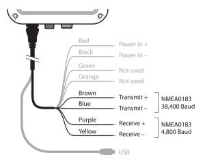
Figure 9 Connecting to the NMEA0183 data port
